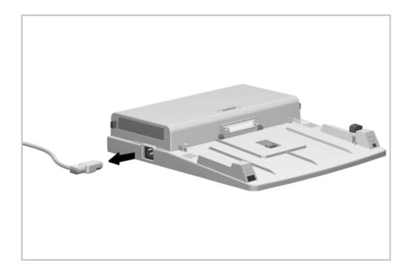
Figure 6-3. Disconnecting the Expansion Base
